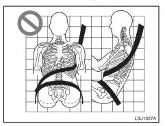
**Answer:** The shoulder belt is worn under the arm. It should be worn over the shoulder at all times.
